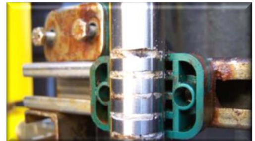
Fig 1 – Tube showing signs of crevice corrosion
