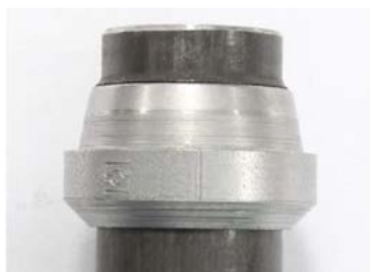
Fig. 17: Result of the cutting ring pre-assembly
