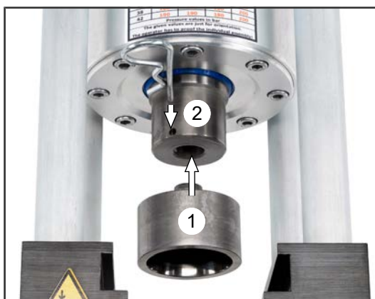
Fig. 8: Assembly stud on the pressure cylinder
