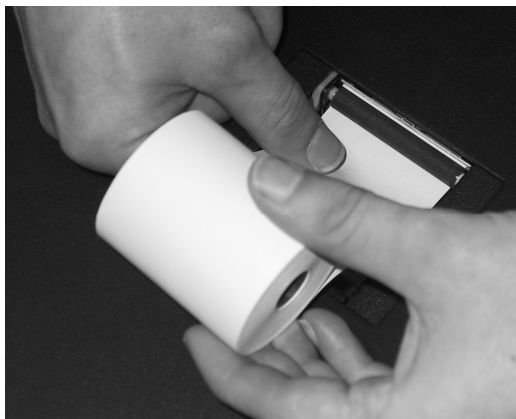
Figure 27: Inserting the printing paper
