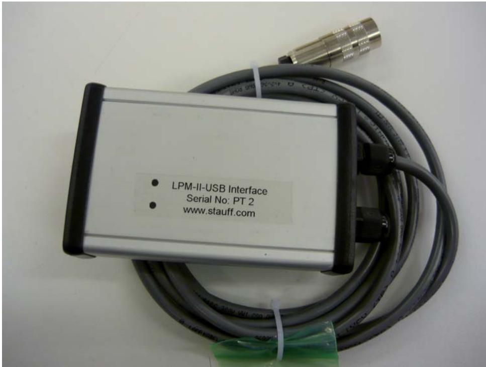
Figure 1 LPMII-USB Interface: A USB Interface Unit for the LPMII
