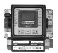
To program the LPT, point the IrDA port on the PDA at the window on the LPT and apply power to the LPT. Enter the configuration mode when prompted. Commonly modified parameters are the N, O, P and H fields.
