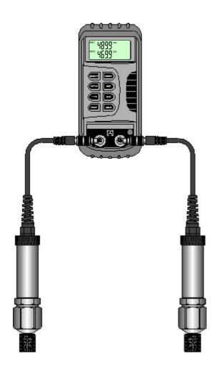
Calibrate the pressure sensors at the operating pressure of the machine.
