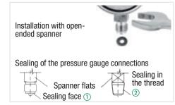
The torque depends on the sealing used. In order to orientate the measuring instrument so that it can be read as well as possible, a connection with clamp socket or union nut should be used.
