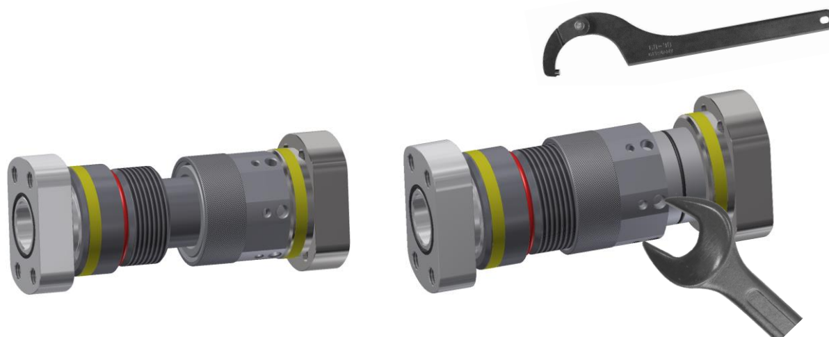
[Fig. 2] Coupling process. Left: positioning the female coupling. Right: Push the threaded sleeve forward and use a tool to tighten to the stop.
