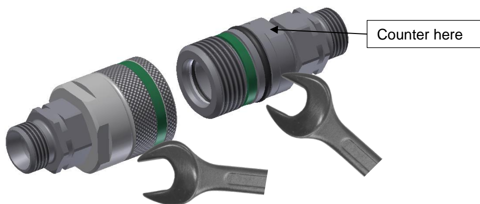
[Fig. 2] Diagram coupling halves: Tighten to the stop with a tool.
