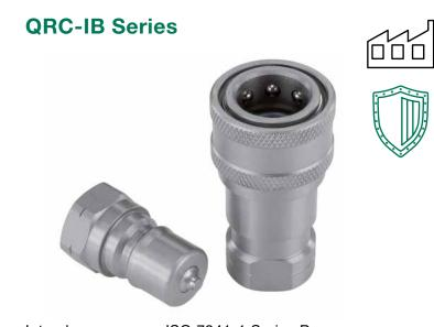
ISO 7241-1 Series B Interchange 1/8" to 2" (DN 3 to 51) 1450 to 7250 PSI Working Pressure Carbon Steel, Brass and Stainless Steel
