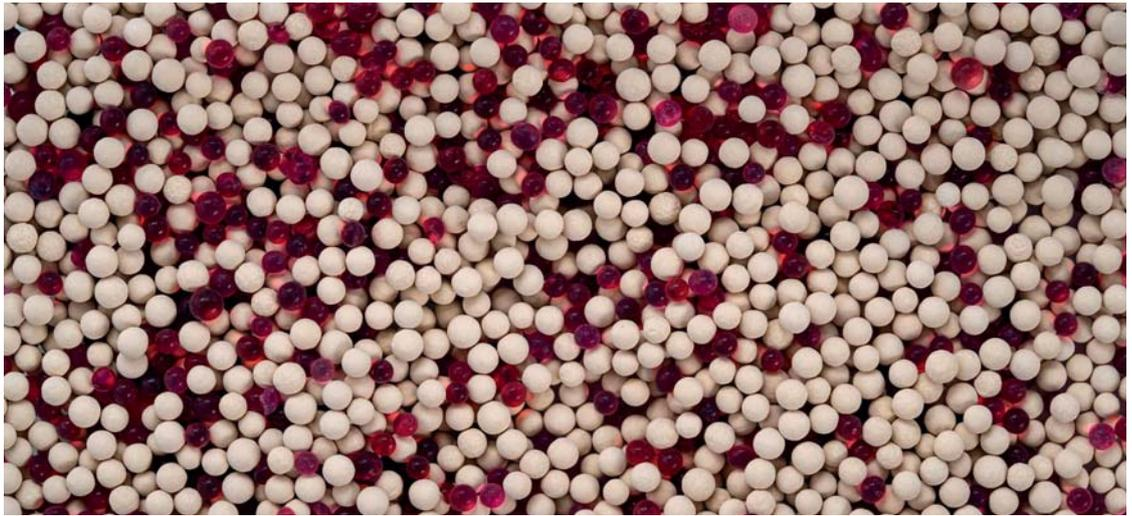
principle is always the same: An initial filter layer separates out the solid particles. The pre-cleaned air flows through a capsule with desiccant before it is then “fine” filtered and discharged into the hydraulic reservoir. The different series in the Stauff desiccant air breather range all have the same water absorption capacity.
