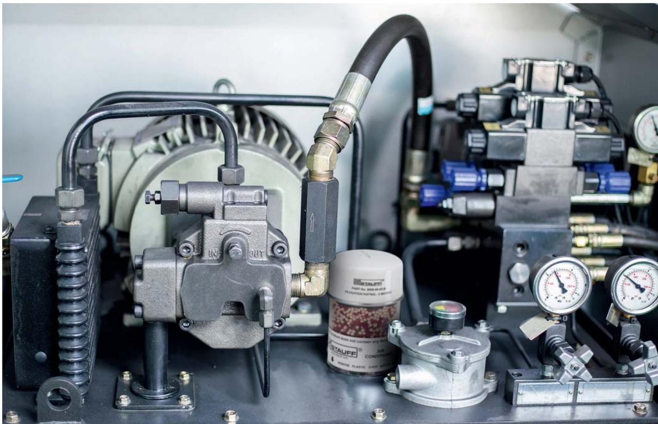
As a part of hydraulic units, giant and desiccant air breathers from Stauff are used in a number of applications in mobile and industrial hydraulics.
