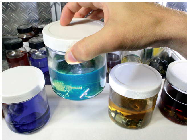
Original equipment manufacturers can also have the coating tested for its resistance to fertilisers, pesticides etc.
