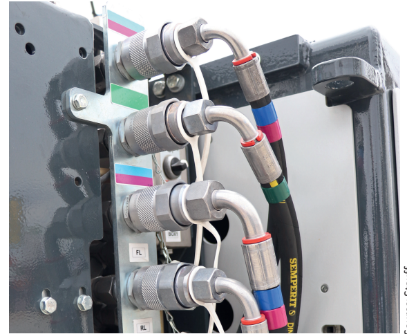
The tube couplings use the principle of screw-to-connect couplings that seal on both sides and have flat-face valve tappets.
