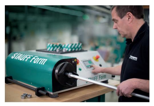
05 The Stauff Form EVO machine shapes the tube end so that a positive connection is created during fitting with a conventional fitting body and a union nut
