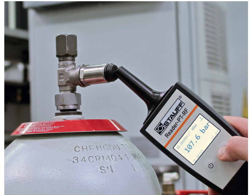
Contactless measurement reduces testing, avoids nitrogen losses, and supports status-based maintenance, stresses Stauff.
