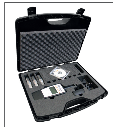
Hydraulic accumulators ensure the stable operation of hydraulic systems and take on central energy and safety functions. However, the correct nitrogen precharge pressure is crucial for the performance, service life, and safety of pressure accumulators. With this complete set from Stauff, the gas pressure can be monitored permanently and without any loss of pressure.
